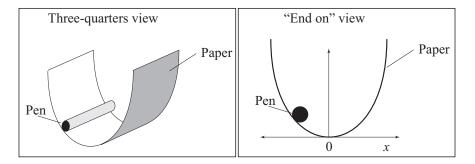
When you do this experiment, the horizontal position of the pen (x in the sketch on the right) is a function of time t, and obeys the following equation (assuming conservation of energy)
